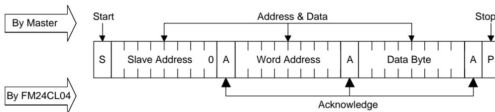
Figure 5. Byte Write
