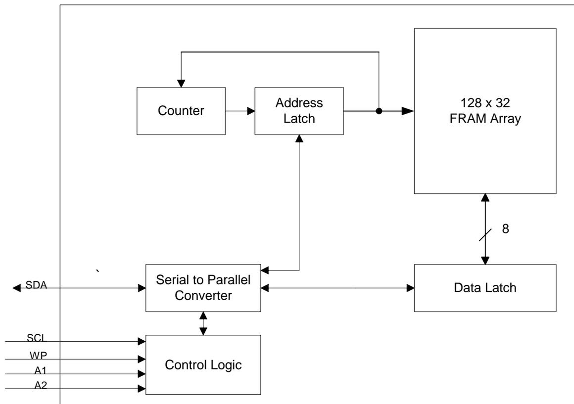
Figure 1. Block Diagram
