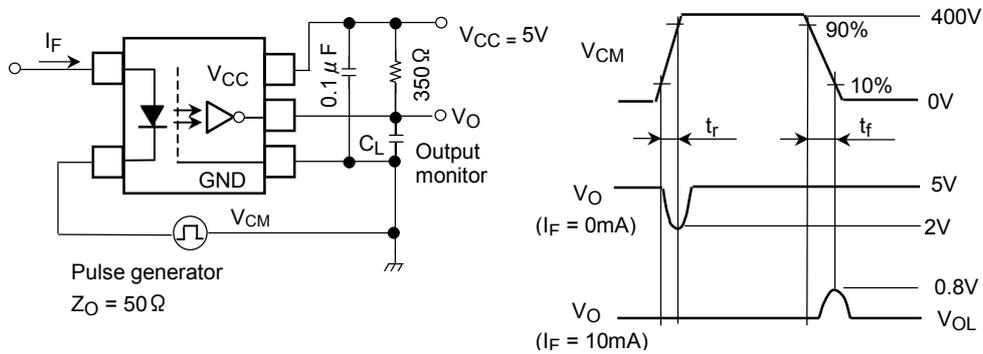
$$CM_H = \frac{320 \text{ (V)}}{t_r \text{ (}\mu\text{s)}}, CM_L = \frac{320 \text{ (V)}}{t_f \text{ (}\mu\text{s)}}$$
