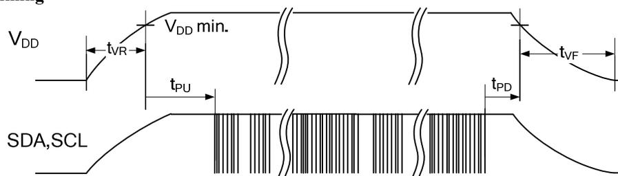
**Power Cycle Timing** ( $T_A = -40^\circ\text{C}$  to  $+85^\circ\text{C}$ ,  $V_{DD} = 2.7\text{V}$  to  $3.65\text{V}$  unless otherwise specified)
