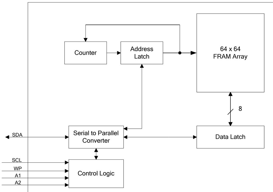
Figure 1. Block Diagram
