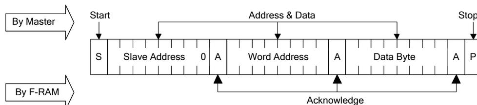
Figure 5. Byte Write
