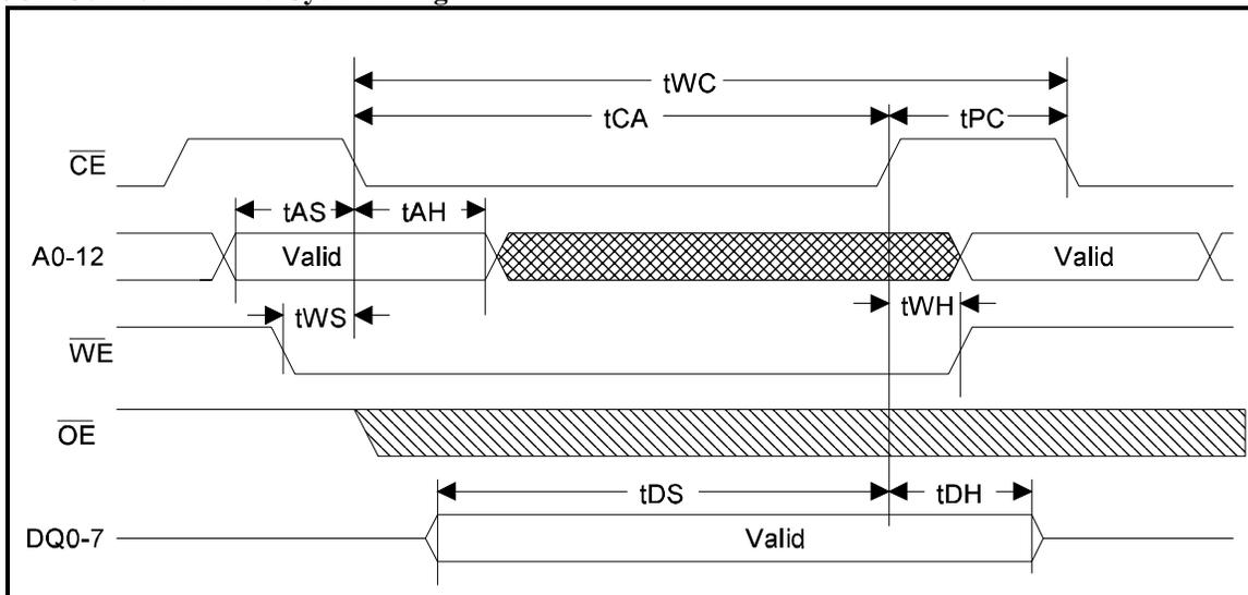
**/WE-Controlled Write Cycle Timing**
